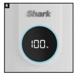
6. When the air purifier power is on, it will begin to analyse the air quality, indicated by the rotating lights.
