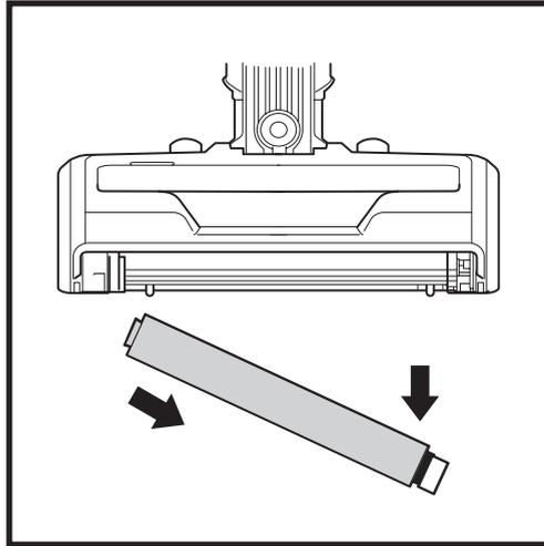
1. Slide **Eject Roller** button forward.
