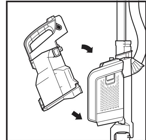
To reinstall the dust cup, place the bottom into the pod and tilt the dust cup toward the wand until it clicks into place.
