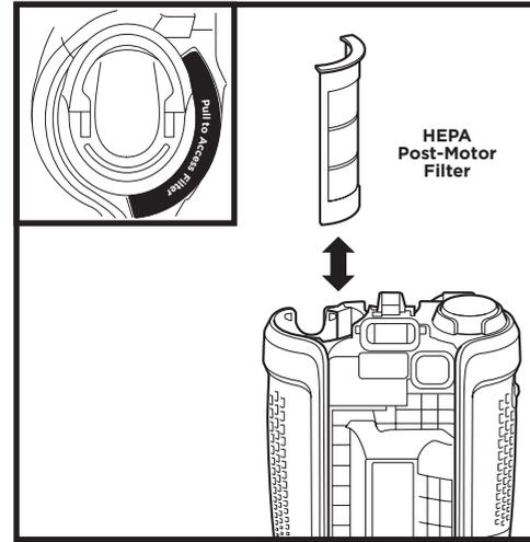
1. Pull up on **HEPA Post-Motor Filter** access tab to remove.
