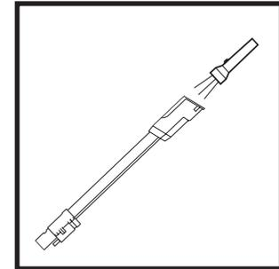
Detach wand from floor nozzle and handle, and check both ends of wand for blockages.
