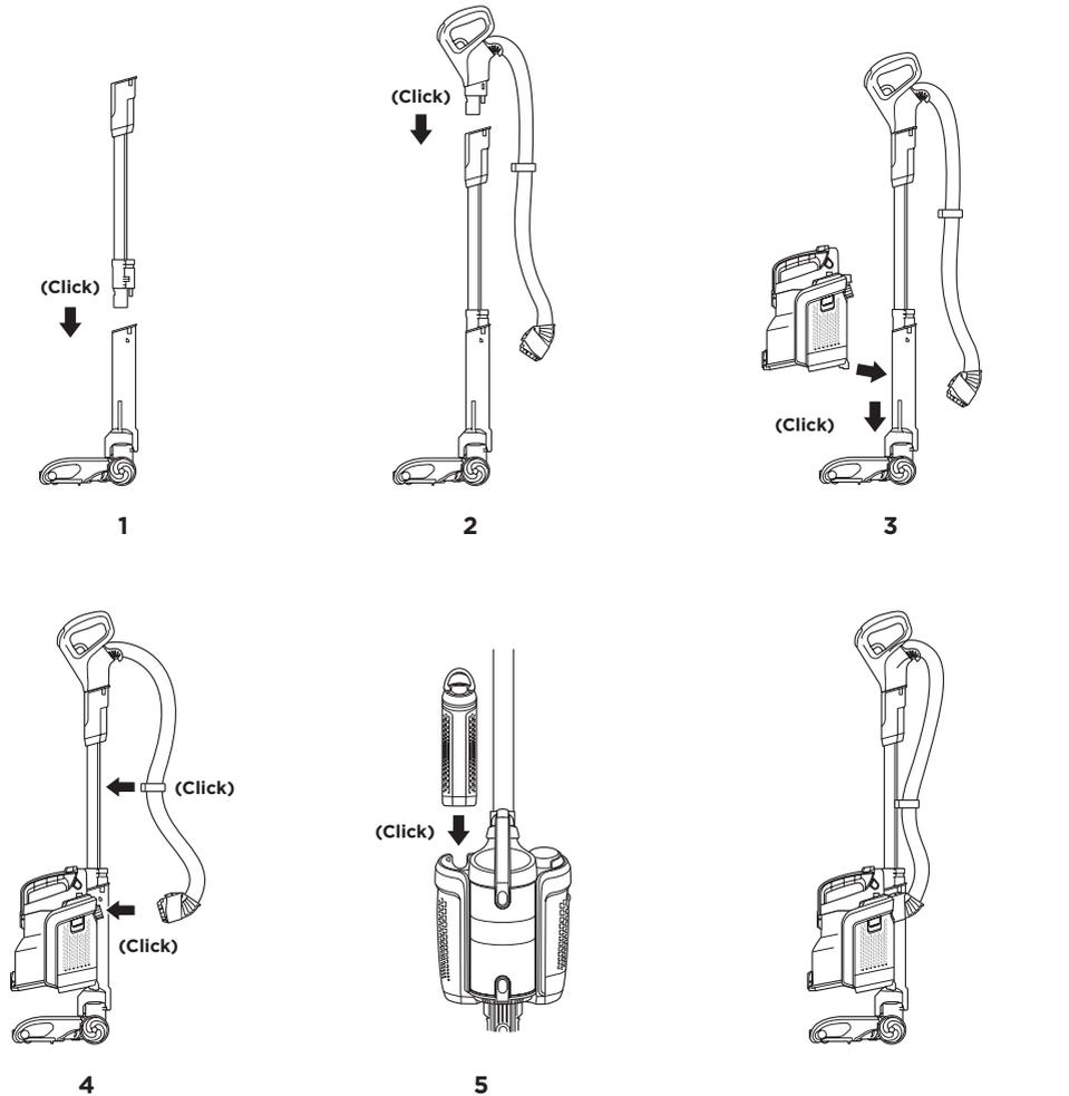
1. Insert the **Wand** into the **Floor Nozzle**.
