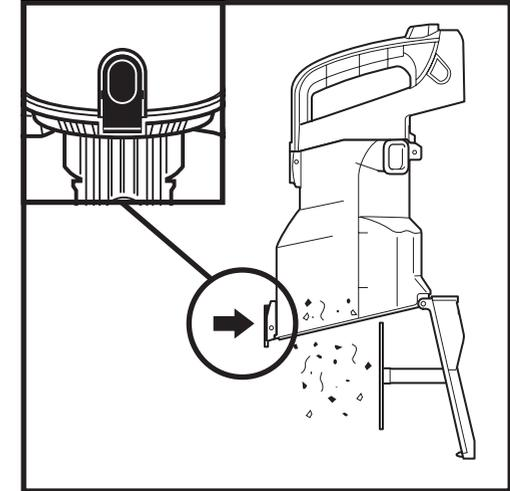
Position the dust cup over the trash, then press the bottom button to release dust and debris.
