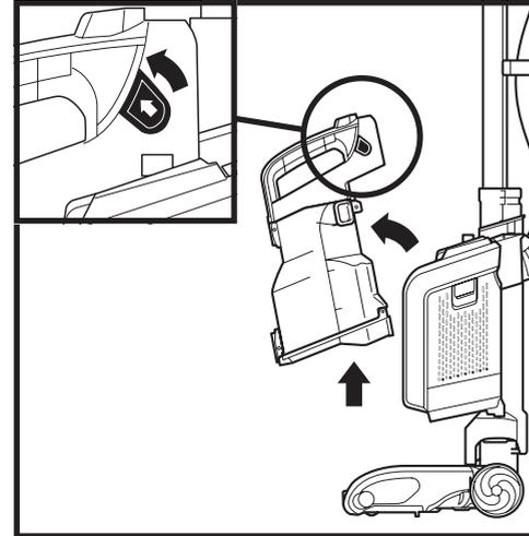
To remove **Dust Cup**, slide up the release tabs on both sides. Tilt the dust cup away from pod, and lift to remove.
