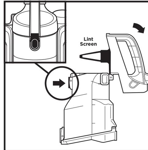
To access the **Lint Screen** inside the dust cup, press the top button and lift the handle to open the dust cup. Brush the screen lightly to remove collected debris.
