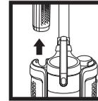
**IMPORTANT:** Remove the battery before performing any maintenance. To remove, lift the handle on top of the battery and pull up.
