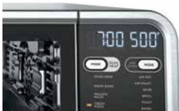
Install high-density pan in the bottom level of the unit, then close door. Select FRESH PIZZA, set temperature to 500°F, and set time to 7 minutes. Press the setting dial to begin preheating.
