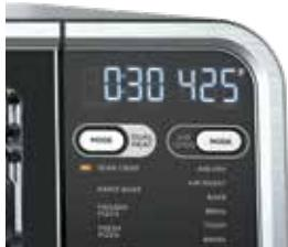
Install the high-density pan in the bottom level of the unit, then close door. Select SEAR CRISP, set temperature to 425°F, and set time to 30 minutes. Press the setting dial to begin preheating.
