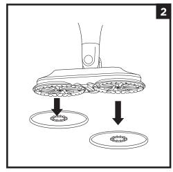
2 To attach the Dirt Grip pads, place **BOTH** the pads flat on the floor with the plastic rings facing up. Align the indentation on the rotating discs on the bottom of the nozzle with the plastic rings on the pads, then gently lower the nozzle onto the pads, pressing until the pads are secured.
