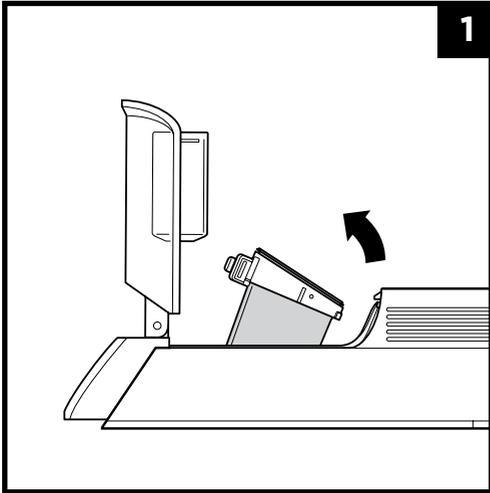
1. With the dust cup removed and the power off, pinch both sides of the filter housing and pivot it upward to access the filter.
