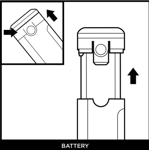
To remove the battery from the hand vacuum, press the release tabs on the battery cap and slide out the battery. To reinstall, slide the battery into the compartment in the handle until it clicks into place.
