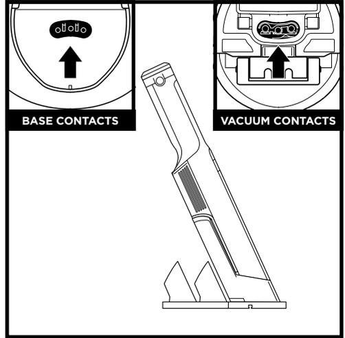
Make sure the contacts on the wand are aligned with the contacts on the charging post.
