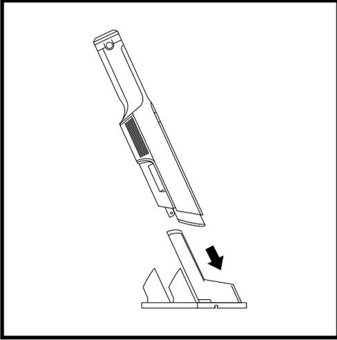
Charge the unit by sliding it into the charging base nozzle-first.
