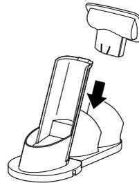
1. Slide the **Onboard Accessory Storage** onto the back of the **Charging Base** until it clicks into place.
