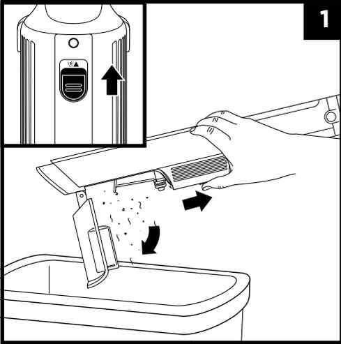
1. With the power off, slide the **Dust Cup** release button on the back of the vacuum towards you, and the dust cup will swing open. Tap the filter screen lightly to knock off dust and debris.
