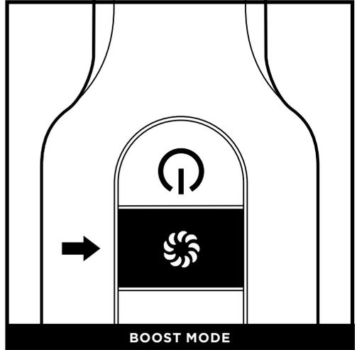
For an added boost of power, press the **Boost** button. Press again to return to normal power.
