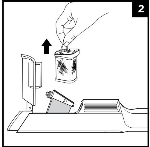
2. Hold the filter housing over a bin. Lift the fabric filter by the metal ring to remove it from the housing. Tap lightly to remove any dust and debris, then rinse with water only. Let the filter air-dry for at least 24 hours or until completely dry before reinstalling.
