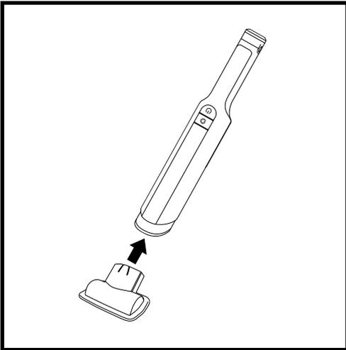
To attach an accessory to the hand vacuum, slide it into the opening in the nozzle. To remove the accessory, slide it off the nozzle.
