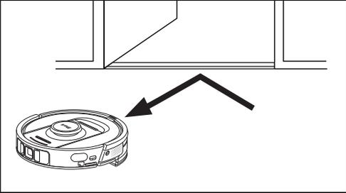
Your robot can easily climb over most thresholds, but if one is higher than 2.5cm, set up a no-go zone in the app to block it off.
