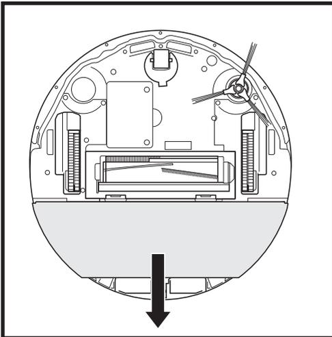
1. To remove the pad plate, use two fingers to gently pull the pad plate off the bottom of the robot.
