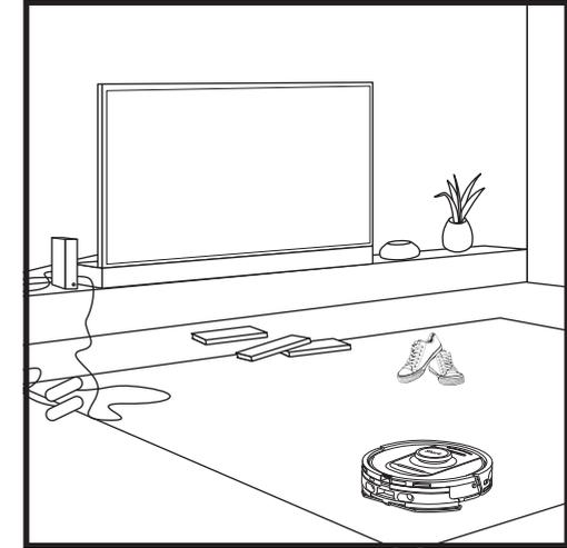
The robot's object detection technology helps it navigate around obstacles taller than 11.5cm in height, as well as some common household objects like cords, cables, shoes, and clothes.
