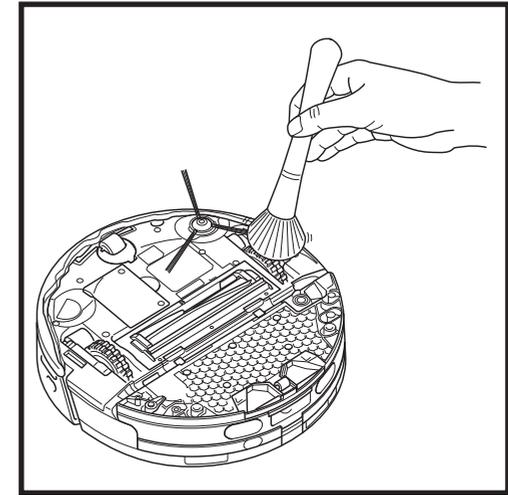
2. Periodically clean the drive wheels and the housing around them. To clean, rotate each drive wheel while dusting.
