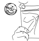
4. Align the yellow arrow on the side of the cartridge with the yellow arrow on the side of the dial cover, then insert the cartridge into the dial. Rotate the cartridge clockwise to lock it in place.
