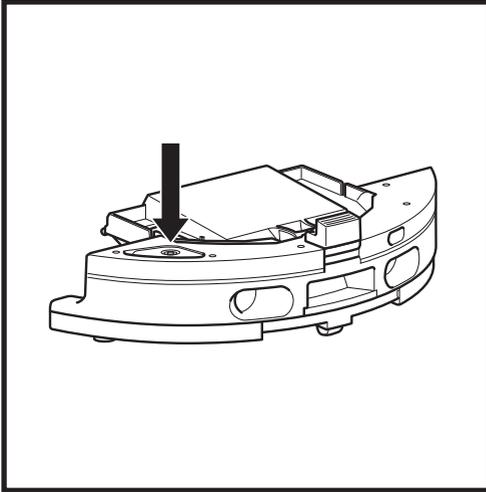
1. To open the robot water tank, pull the rubber stop from its sealed location to open the port. Fill with water and then secure the rubber seal back in place.
