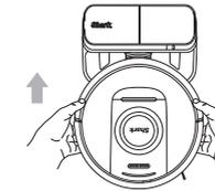
1. **Align the robot with the Shark logo upside down, then slide it up the ramp, onto the base.**
