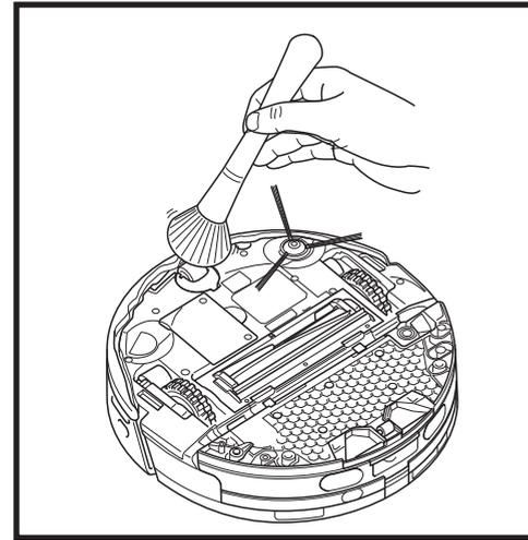
1. Rotate the front wheel while lightly brushing away dirt and debris. Clean the wheel and the housing around it.
