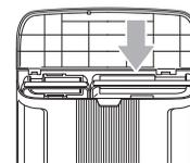
1. Lift the water tank off the front of the base.
