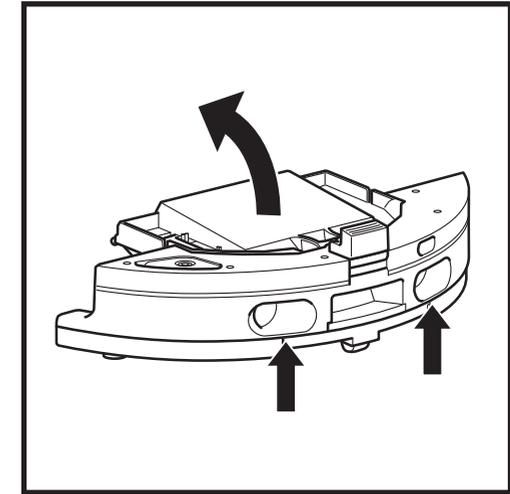
To open the robot dust bin lid, pinch and lift up using the finger slots.
