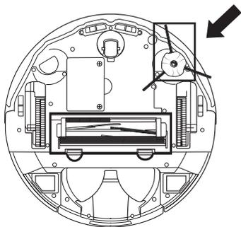
Attach the side brush to the post on the bottom of the robot.
