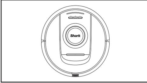
If your **POWERDETECT** Base has enough water in the clean water tank and has a pad plate with mop pad attached, you can begin a wet clean by simply pressing **WET** icon
