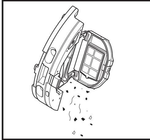
2. Every time you empty the dust bin, slide the filter out and lightly tap it over a trash can to remove any dust and dirt. Use a dry cloth or soft brush to remove any remaining debris.
