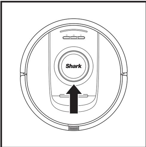
1. Check the navigation module on top of the robot and gently remove any hair or debris.
