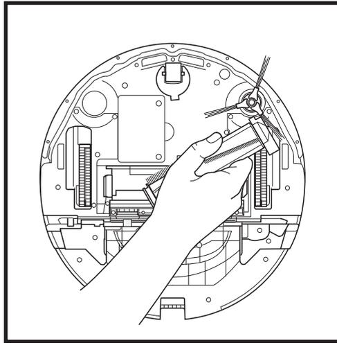
2. Take out the brushroll and remove the cap on the end. Clean off any hair or debris then replace the cap. Reinstall the brushroll, inserting the flat end first. Close the brushroll access door and press down until both sides click into place.
