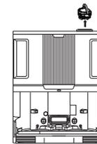
2. Rotate the cartridge anti-clockwise in the dial housing and pull out the cartridge to remove it.
