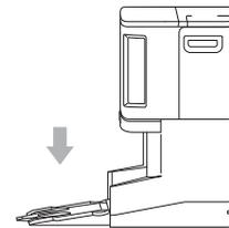
1. Align the flat side of the ramp with the bottom of the base.
