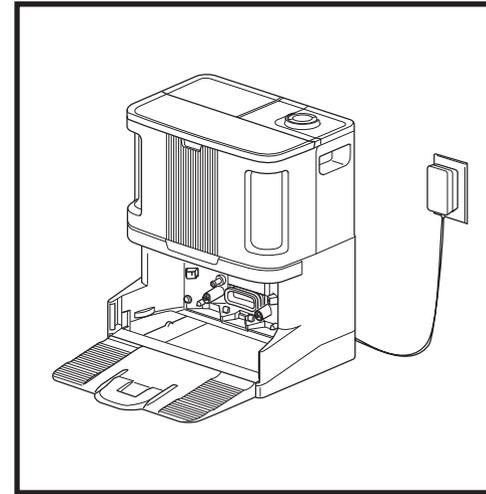
With the ramp removed, you can access the pad plate tray.
