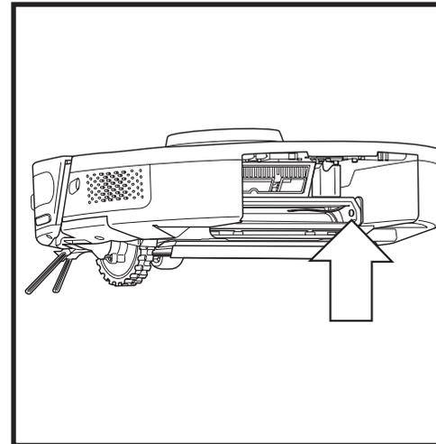
Remove the robot dust bin. Using a dry microfibre cloth, wipe off the area indicated to remove any dust or debris covering the sensor.
