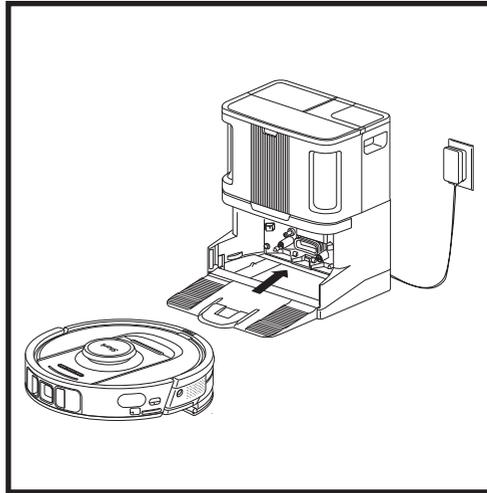
When the cleaning cycle is complete, or if the battery is running low, the robot will search for the Self-Empty Base. If the robot doesn't return to the base, its charge may have run out.
