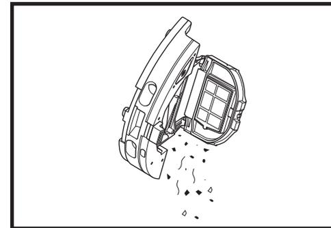
Empty debris and dust into the trash. If desired, you may use a dry cloth to wipe the interior of the dust bin.
