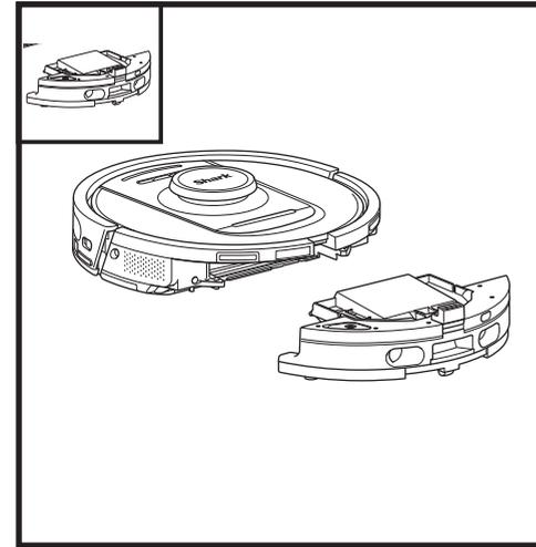
Press the **Dust Bin Release Button** and slide the dust bin out from the robot.
