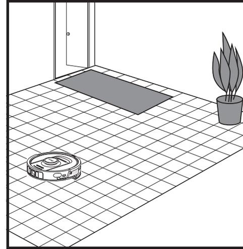
After setup is complete, your robot will conduct an **Explore Run** to create an initial map of your home. The robot will travel from room to room to identify walls, furniture, carpets, and other obstacles as it cleans. The robot will complete a full dry clean as it creates the map of your home.
