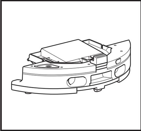
1. Remove and empty the dust bin. Clean any hair or debris off the back of the dust bin.
