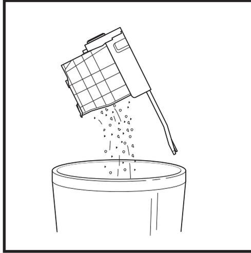
To empty the bin, hold it over the trash, then press the dustbin release button to empty. The bin lid will open, releasing dust and debris. Lightly tap the dust bin against the inside of the trash receptacle to knock off any remaining debris. Reinstall the bin by sliding it into the slot in the base until it clicks into place.
