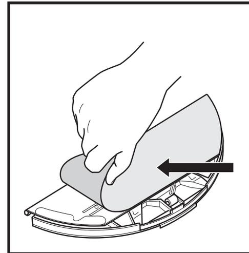
3. Slide a clean or new pad into the edge of the pad plate. Secure the pad to the plate with a light press to engage the Velcro.
