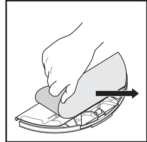
2. Slide the pad to one side, away from the pad plate.
