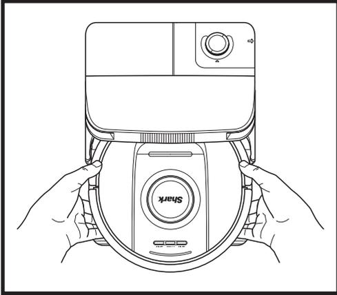
To **TURN THE ROBOT ON:** Slide the robot up the ramp on to the base or hold down DOCK icon
