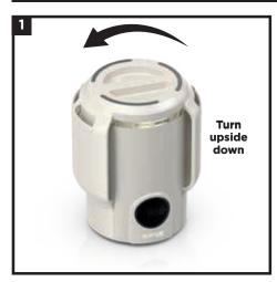
1. DO NOT plug in the air purifier. First, carefully turn the air purifier upside down and place it on a level, floor surface. Rotate the filter door counter clockwise to the unlocked position to access the HEPA filter.
