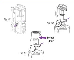
IMPORTANT: Loss of Suction may occur if foam filters are not cleaned every 3 months. Rinse and allow to air dry completely. Foam filters may appear dirty after use - this is normal.
