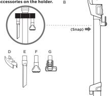
Lift the floor nozzle tube, pushing it firmly until it stands upright, then insert the wand into the tube.
