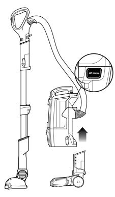
3 Press the LIFT-AWAY button to lift the pod off the motorised floor nozzle.
