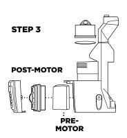
**3** Remove the filter assembly, then remove the pre-motor filter from the assembly. Rinse both filters and allow to air dry completely before replacing. Hand wash only.
