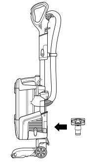
**3** Place pod onto wand and slide down to connect. 4 Connect hose into back of pod, pressing it in until it clicks securely into place.
