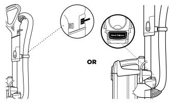
**1** Press the Handle Release button to clean above-floor areas with the handle.
