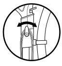
TIP: Use cord clip located on the side of wand to hold cord in place while vacuuming.
