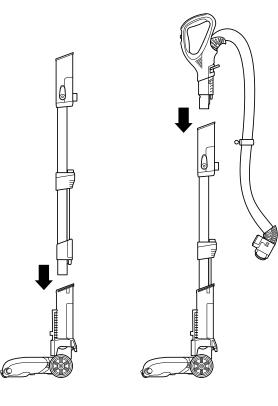
1 Place motorised floor nozzle on floor and insert wand, pressing it in until it clicks securely into place.
