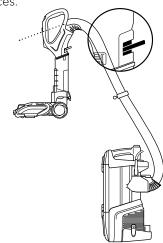
**2** For a convenient way to clean stairs, remove the wand and insert the handle into the motorised floor nozzle.
