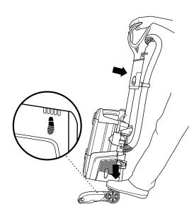
1 Plug power cord into outlet. Place foot on floor nozzle and tilt handle back.
