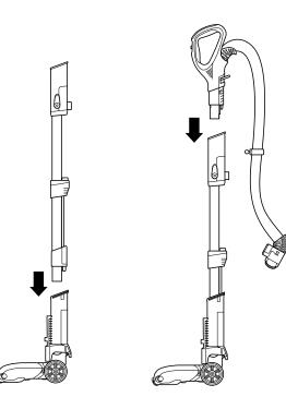
1 Place motorised floor nozzle on floor and insert wand, pressing it in until it clicks securely into place.
