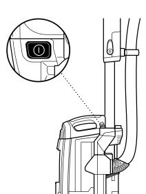
2 To start cleaning, press power button to turn on vacuum. Please note the brushrolls will not spin unless the unit is reclined.
