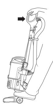
1 Plug power cord into outlet. Place foot on floor nozzle and tilt handle back.
