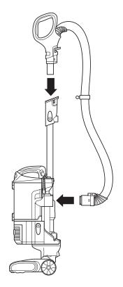
hose to hose connector on base of pod.
