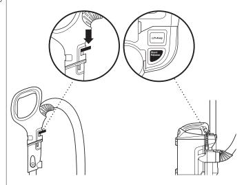
1 To clean within short reach, push handle latch down, then lift the handle up off of the wand.
