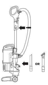
3 Insert handle into top of wand. Then attach 4 Insert tools into accessory holder, then secure the hose to the hose clip by pushing the knob into its socket.
