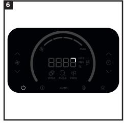
**6.** When the unit is powered on, it will begin to analyse the air quality indicated by the rotating lights. After a few seconds the unit will display the current air quality and you can customise the settings on your unit.
