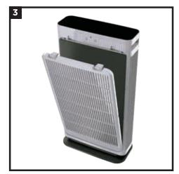
3. With the filter installed, replace the filter cover. Insert the tabs on the bottom of the cover into the slots on the unit. Press the top of the cover, then the sides, until it clicks into place. DO NOT run the air purifier unless the filter is removed from its packaging and installed correctly.
