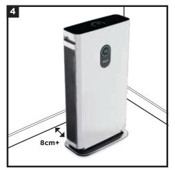
**4.** Set up the unit upright on a level floor. For best results, set it up in the space you spend the most time in, such as the kitchen, living room, or bedroom. Make sure the unit is at least 3 inches (8cm) away from all walls, large objects, or electronics.
