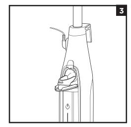
**3** To open the water tank, pull the lid down. Unplug the steam mop before refilling the water tank.
